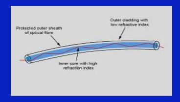
When an ray of light travels from a denser to a rarer medium such that the angle of incidence is greater than the critical angle, the ray reflects back into the same medium this phenomena is called TIR.
